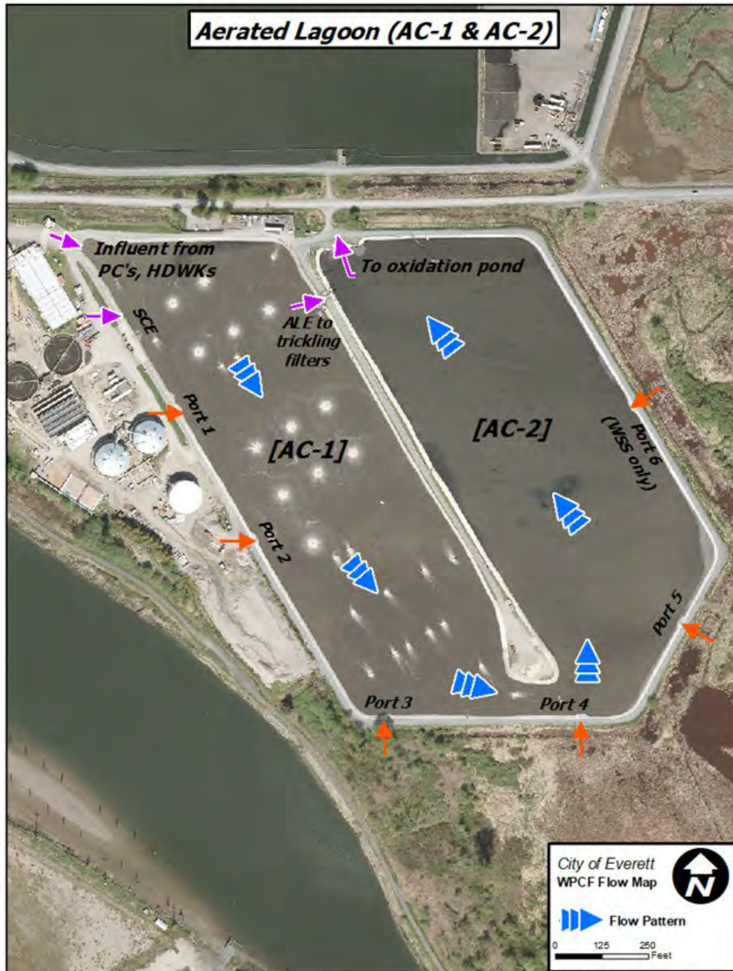
Figure 1 - Aerated Lagoons Flow Diagram
